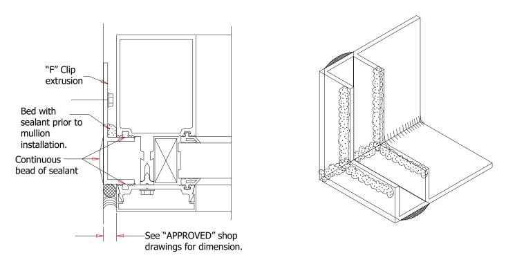
Perimeter With Continuous "F" Extrusion.
