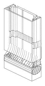
Caution: Care must be taken to avoid damage to covers during installation. Use a nominal 12" long, 2" X 4" block, and mallet or hammer to seat cover.
