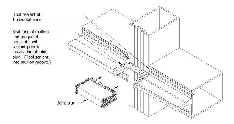
Note: All sealant shown on this detail must be done just prior to installation of joint plug. Keep free from loose debris. <u>Seal of Horizontal to</u> <u>Mullion and Joint Plug</u> <u>at "Stack" Horizontals</u>
