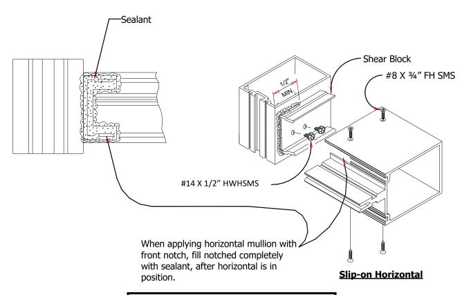
Note: When using slip-on horizontal, 2 screws are required on top and bottom of horizontal into the shear block.
