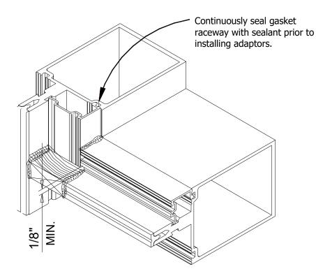
Note: Vertical adaptors will need a minimum of 1/8" clearance above joint plug, free FROM sealant.
