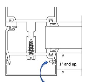
On horizontals, (2) 1/16" X 5/16" Roll Pins need to be located on top side (when possible) of horizontal and place between 1/4 and 1/3 points of D.L.O.
