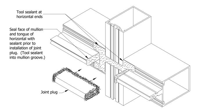
Note: All sealant shown on this detail must be done just prior to installation of joint plug.
