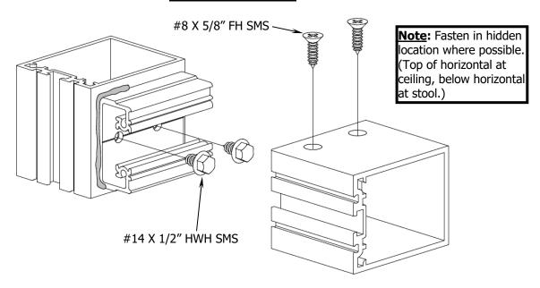
Note: Level shear block before fully tightening screws
