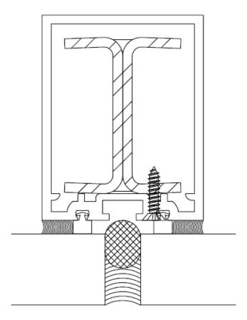
D.) When steel reinforcement is factory installed in mullions, fasteners will be used to prevent damage or slippage of steel during shipment
