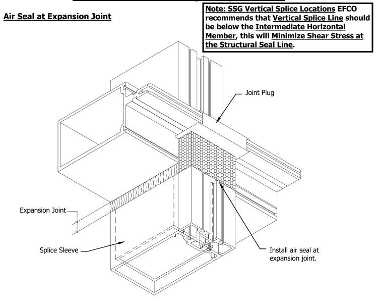
Note: At corners, use more than one air seal as required. Miter to fit corner.
