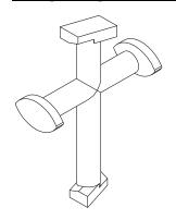
**Silicone Structural Glazed Temporary Retainer**
