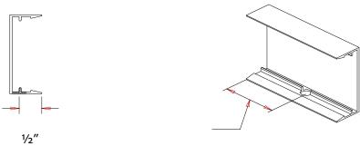
Drill 5/16" diameter weep holes in horizontal covers at 2" from vertical covers.
